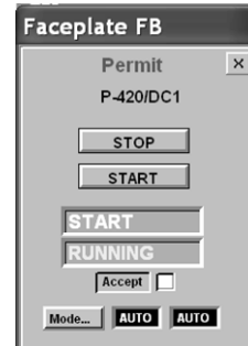
Figure 7. Faceplate for control pump P-420.
