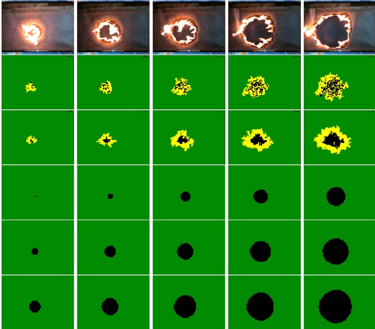
Figure 2. Top panel: A sequence of observed burn patterns for a fire on a sheet of wax paper (at 0 slope) observed at 1 second intervals. Time increases from left to right. Second and third rows: Realizations of simulations of Models A and B under homogeneous conditions with \mu = 0.2 , \lambda_N = 1.336 , \lambda_S = 1.312 , \lambda_E = 0.896 , and \lambda_W = 1.424 , observed at approximately 1 second intervals. Both models were simulated on a 60 x 75 grid. Third row: A realization of a simulation of Model B under homogeneous conditions with \mu = 0.2 , \lambda_N = 1.336 , \lambda_S = 1.312 , \lambda_E = 0.896 , and \lambda_W = 1.424 , observed at approximately 1 second intervals. Both models were simulated on a 60 x 75 grid. Fourth row: Black area represents regions which burned in at least 90% of 1000 simulation runs. Fifth row: Black area represents regions which burned in at least 50% of 1000 simulation runs. Bottom row: Black area represents regions which burned in at least 10% of 1000 simulation runs.
