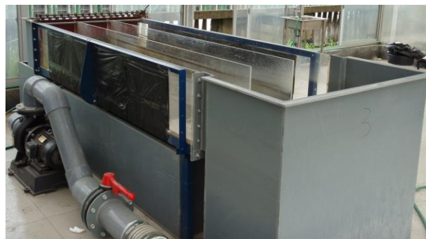
Figure 1. Overview of the experimental setup in one treatment. Water in the lower reservoir is pumped into the right basin. Overflowing water is moved to the left basin through the flumes which contain the experimental sediment/water interface. The hydrodynamic force comes from a water pump with a max flow of 100 m 3 /h.
