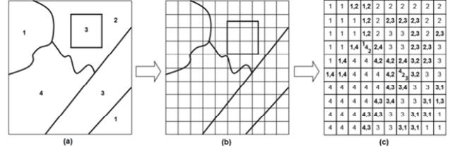
**Figure 4.** Conversion of a vector map to a raster: (a) vector dataset containing polygons with associated labels; (b) a grid with the desired cell size; (c) the values of the grid cells become the values of the labels of the polygons which contain them.
