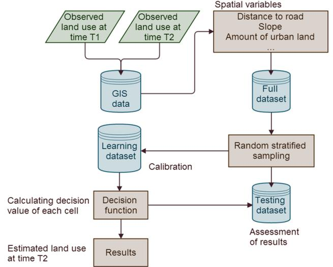
**Figure 2.** Flow chart of the procedure for modelling land-use change using the DML $k$ NN method.
