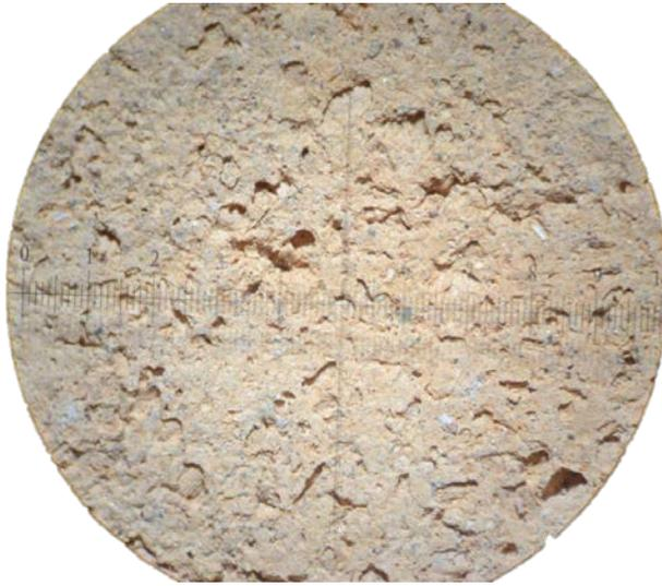
**Figure S3.** Microscopic image of CWF surface: 1mm field of view (Keyence VHX-5000 digital microscope).
