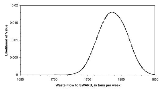
**Figure 1**. Scenario 1: weekly distribution, in tons per week, of SWARU use for the best solution found when it must be operated within its maximum operating capacity range of [2500, 2700] tons per week, but may violate this requirement 10% of the time.
