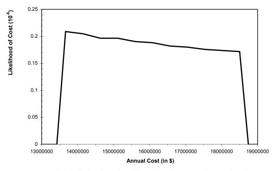
**Figure 8**. Scenario 3: distribution of annual costs best solution when SWARU is operated anywhere in the range between being closed completely up to its maximum operating capacity.
