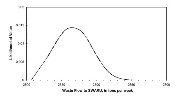
**Figure 2**. Scenario 2: Weekly distribution, in tons per week, of SWARU use for the best solution found when the incinerator must be strictly operated within its maximum operating capacity range of [2500, 2700] tons per week.
