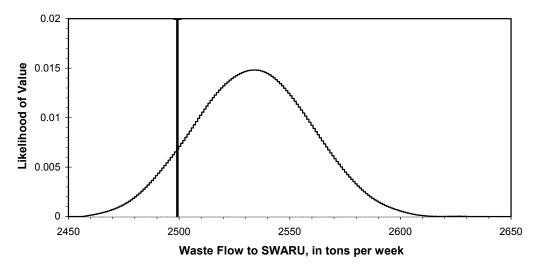
**Figure 5**. Scenario 2: weekly distribution, in tons per week, of SWARU use for the best solution found when it must be operated within its maximum operating capacity range of [2500, 2700] tons per week, but may violate this requirement 10% of the time.
