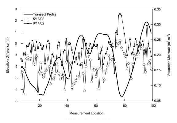
**Figure 2**. Moisture patterns for two days in relation to an exaggerated longitudinal profile (solid line, left axis) of studied transect.
