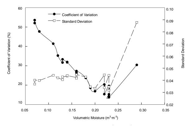
**Figure 4**. Daily mean moisture variability showing standard deviation from the daily mean and coefficient of variation vs. increasing mean moisture measurements.
