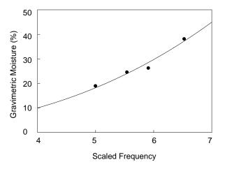
**Figure 1**. Capacitance probe calibration curve for a single location with scaled frequency versus gravimetric moisture sampled on four different days ( $R^2 = 0.96$ ).
