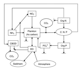
**Figure 3**. Structure of the EUTRO sub-model of the WASP software (Ambrose et al., 1993).
