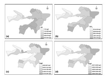
Figure 8. Spatial distribution of a) DO, b)  $NH_3-N$ , c) Org-N, and d) Org-P with 90% reduction in pollutant load and water releases of 1.45 m<sup>3</sup>/s.
