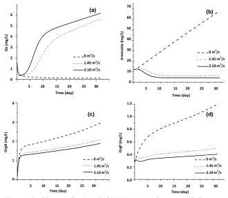
**Figure 7**. Changes in a) DO, b) NH<sub>3</sub>-N, c) Org-N, and d) Org-P in sub-area 4 with different water-release levels.
