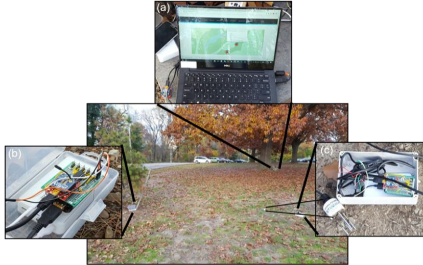
Figure 6. (a) Base Station (Top) setup, (b) End Node 1 (Left) setup and (c) End Node 2 (Right) setup.
