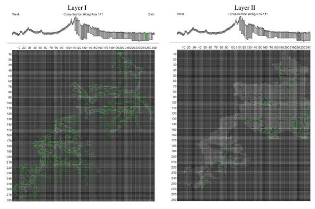
Figure 8. Model boundary conditions in modeled layers. Green color marks block with condition III (river), dark gray color marks blocks with condition II (Q = 0).
