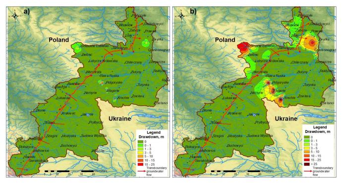
Figure 13. Simulated drawdown (m) in the Bug–San MEA caused by two exploitation scenarios: a) - Scenario II (current exploitation) and b) - Scenario III (maximum permitted exploitation).
