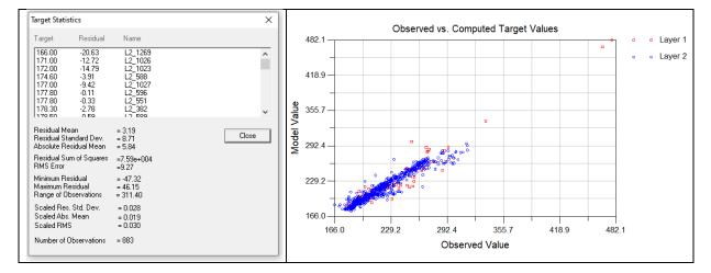
Figure 9. Observed vs. calculated groundwater tables.
