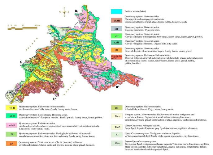
Figure 2. Geological map of the study area and lines of hydrogeological cross-section shown in Figure 3 (line BB") and Figure 4 (line CC").
