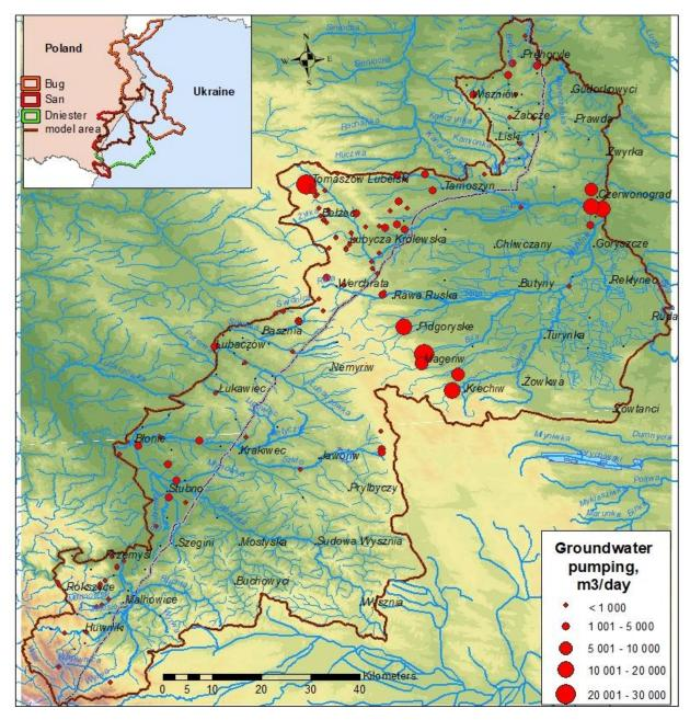
Figure 11. Maximum allowable groundwater pumping for operating intakes (Scenario III).
