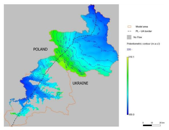
**Figure 12.** Hydraulic head contour lines of the main exploitation aquifer (Layer 2) for the current state (Scenario II - Average daily consumption of groundwater in the operating intakes, 2018 ~ 2021).
